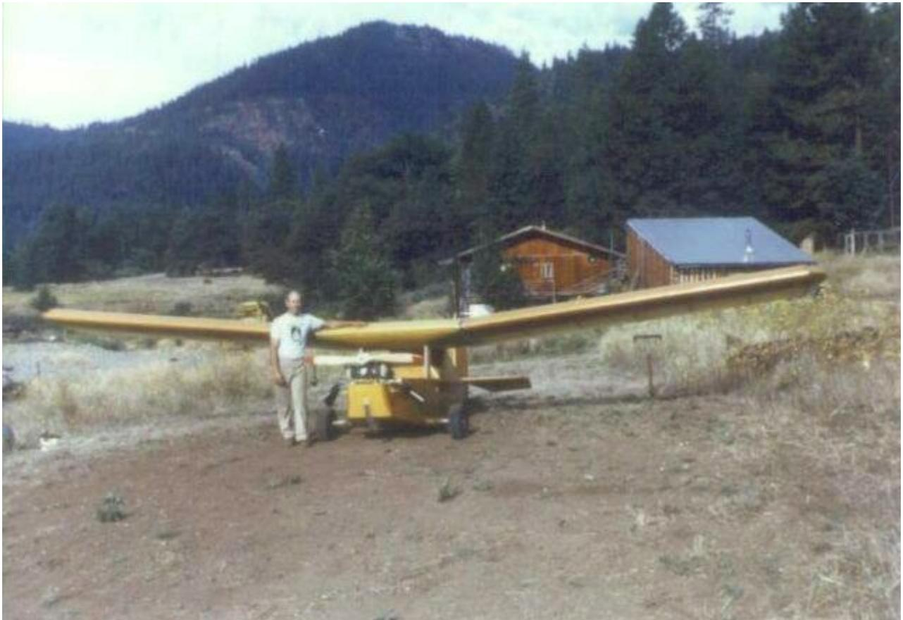
Shown above is the yellow Sky Pup built by Brian Helsaple from Seiad Valley, CA. The engine is a highly modified 1969 Rotax 377 opposed twin cylinder. The bulky air cooling shroud and flywheel were drastically remodeled with a hacksaw and file. Cylinder heads were no longer available so two Yamaha heads were modified to fit. Also, no parts were available for the pull starter so he fabricated
