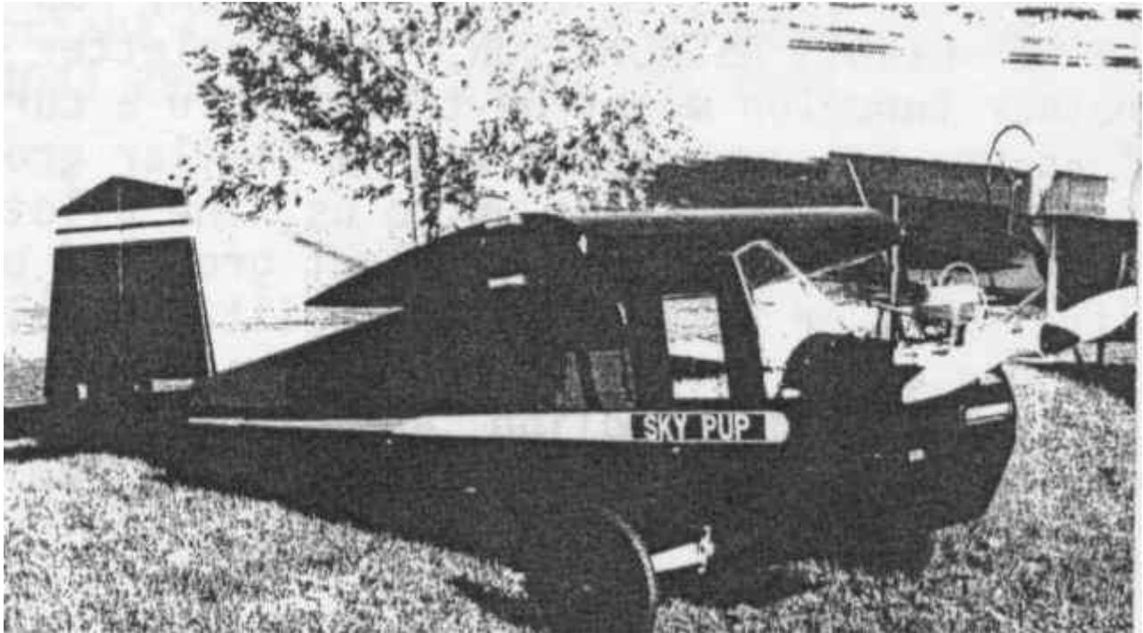
Donald Diggs of Monon, IN reports that his Rotax powered Pup is nearing completion. the color is Navy blue with white trim. Unique features include a foam and plywood engine cowl with windshield and a 2 gal. aluminum fuel tank installed behind the main spar under the centersection shear panel. He hopes to be flying by early next spring. We live only 100 mile apart so we may fly together someday
